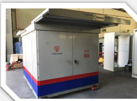
Development of TNB Compact Sub-Station (Tenaga Nasional Berhad)
