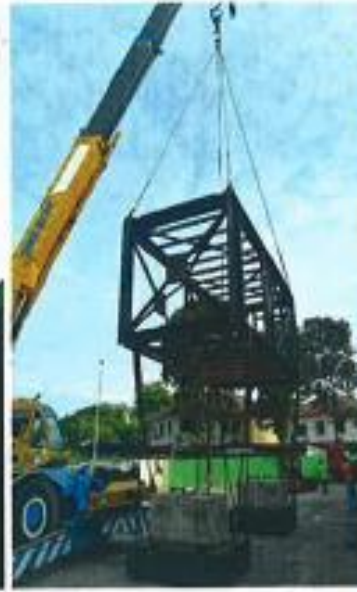
LOAD TEST WORK IN PROGRESS & HOLDING TIME : 10 MINUTES.
