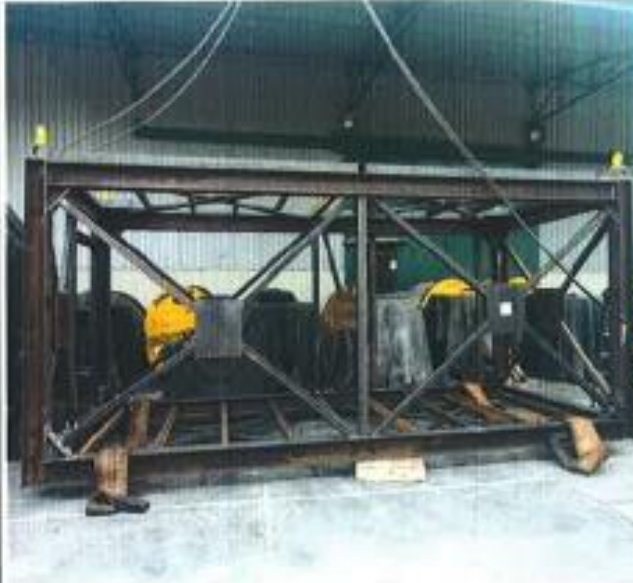
E HOUSE FRAME CONTAINER. TARE WEIGHT – 5TON
