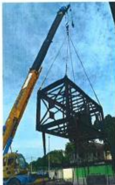
LOAD TEST WORK IN PROGRESS & HOLDING TIME : 10 MINUTES.
