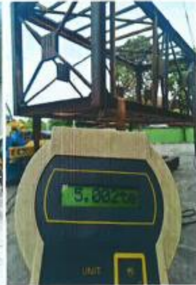
E HOUSE FRAME CONTAINER. TARE WEIGHT – 5TON
